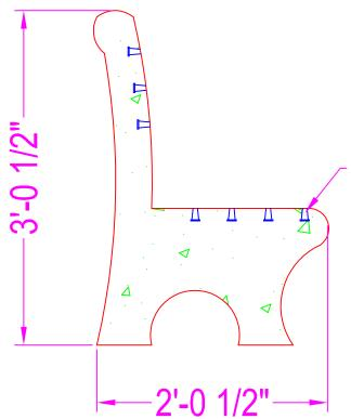
Threaded Inserts Cast in Concrete for Anchoring 2" x 4" Lumber
