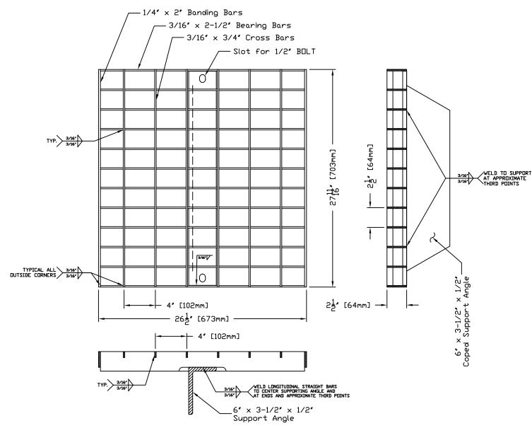
3/16' x 2-1/2' BEARING BARS SHALL BE HOT ROLLED STEEL CONFORMING TO ASTM A1011.
